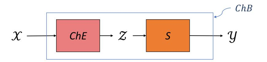
**Degradation**: *ChB* is a degradation of *ChE* if and only if Eve can perfectly simulate *ChB* using *ChE*.
